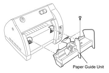
**4.** When changing the media to less than 4.2" (106 mm) wide one, install the Paper Guide Unit in the reverse order of removal
